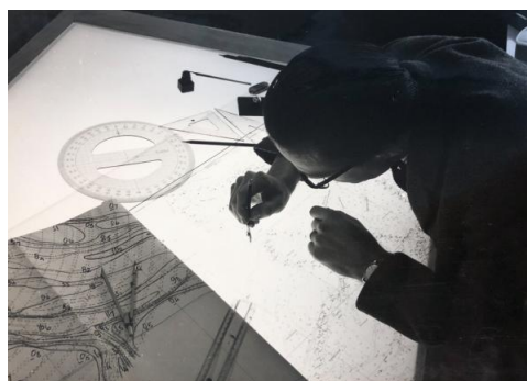
Figure 9. Engraving nautical charts (source: Hydrographic Service)
