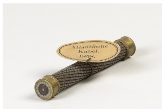
Figure 1. Sample of the first trans-Atlantic submarine telegraph cable 1857/1858 constructed by the Atlantic Telegraph Company [Teylers Museum, Inv.Nr. FK 1056.1.002]
